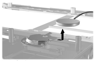
Removing the RTC Battery
